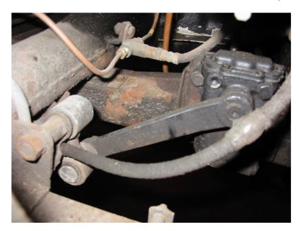
2. \*\*\*\*WARNING Fire Risk\*\*\*\*\* The fuel pump needs repositioning, we recommend extreme care. Remove fuel pump from its existing bracket. .
